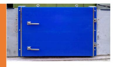
Swing-hinge flood gates provide either flooding protection or chemical containment in bunded areas. The gates are securely sealed with 2 or 3 lever type locking handles. The precision engineered hinges allow the gates to open the full 180° and this can be further extended to 270° with modification.
